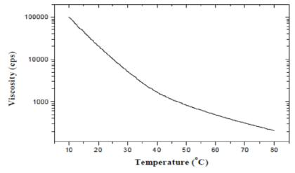
With the increase in temperature the reduction in viscosity is observed, the typical viscosity at temperatures >80°C is < 100 cPs.
